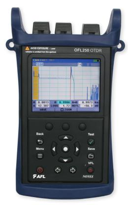
The NOYES OFL250-50 is a 1550 nm single-mode OTDR with an integrated optical power meter (OPM), 1550 nm laser source (OLS), and visual fault locator (VFL) in a hand-held package weighing only 0.8 kg (1.8 lb). With short dead zone and midrange dynamic range performance, the OFL250-50 is ideal for troubleshooting dark single-mode fibers in local access, metro area, and FTTx networks.
